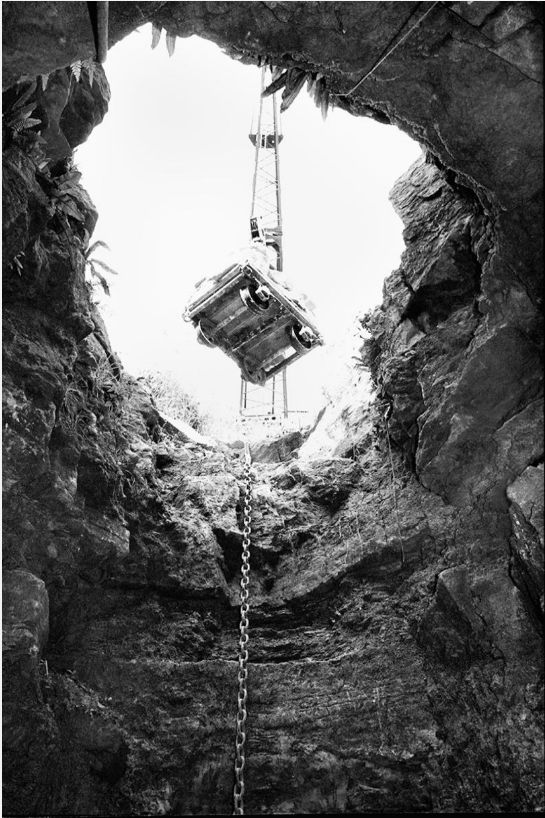
A diesel-powered crane was used to hoist the cart up the vertical shaft.
