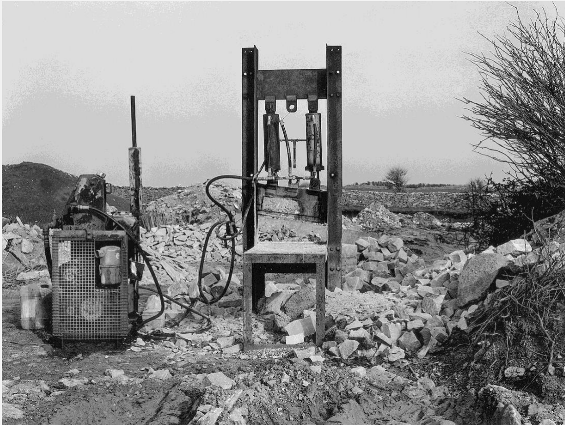
Hydraulic guillotine stone splitter at Alan Landers 1992
